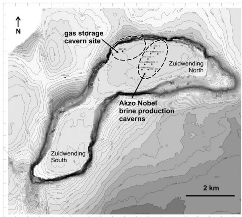
**Figure 1:** Depth contour map of the Zuidwending salt dome structure (top Zechstein Formation, modified from [2]) and general location of the project area.
