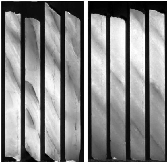
**Figure 4:** Rock salt from the Zechstein 2 (left) and Zechstein 3 cycles (right). Each core piece is approx. 1 m long. Note how thin anhydrite streaks indicate internal structures. Photographs are taken with lighting from behind.
