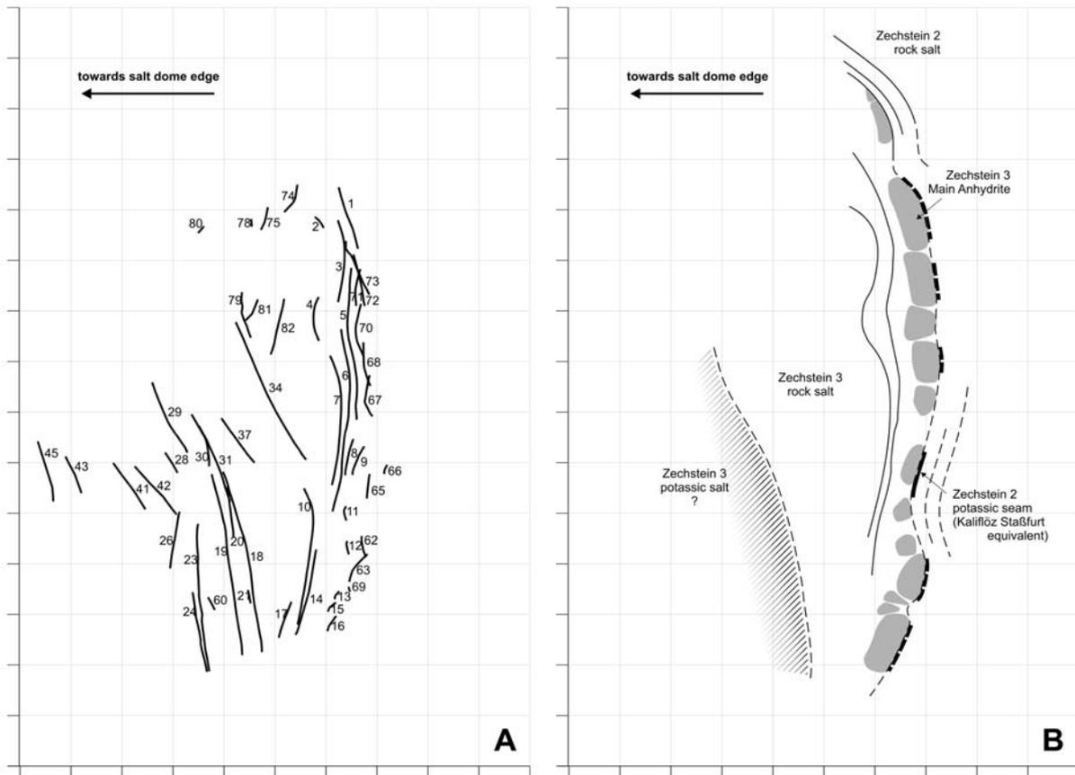
**Figure 3:** GPR data set of more than 40 reflectors with angular information (A) and stratigraphical/structural interpretation (B). Grid spacing is 50 m.
