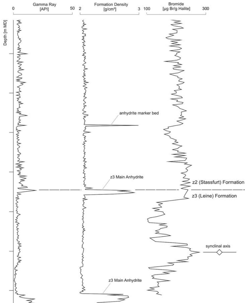
**Figure 2:** Data set of gamma ray and density logs as well as bromide profile for a defined depth interval. The correlation of the curves allows for geological interpretation (each increment of the vertical axis is 200 m).
