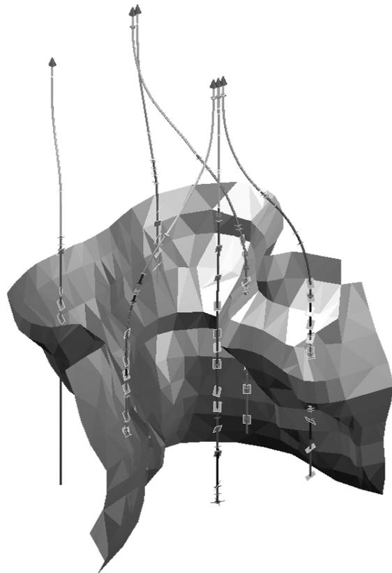
**Figure 5:** Example of a 3D triangulation model of a curtain-like formation boundary plane penetrated by deviated cavern wells.
